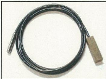
Fig.2 Prototype Fiber Pupil Slicer Unit
